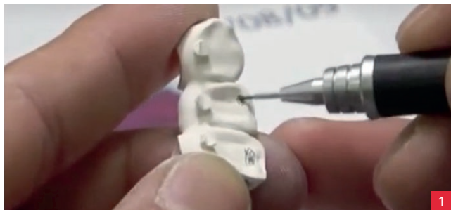
After separating connector, mark areas that are not milled due to undercut.
