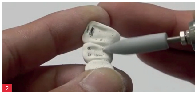
Remove marking area using a silicone bur.
