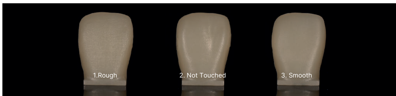
Tidy up the surface using the wheel for zirconia.
